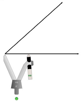
Step 3 On original measure out "new radius" which the length between 2 point of intersection of arc.
